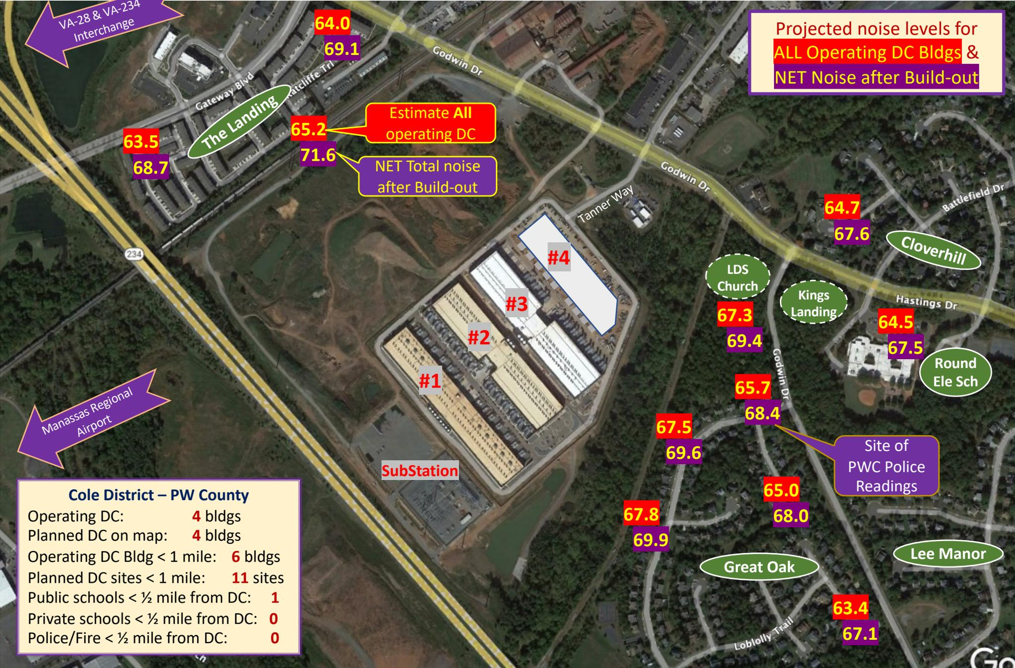
Projected noise levels for ALL Operating DC Bldgs & NET Noise after Build-out
