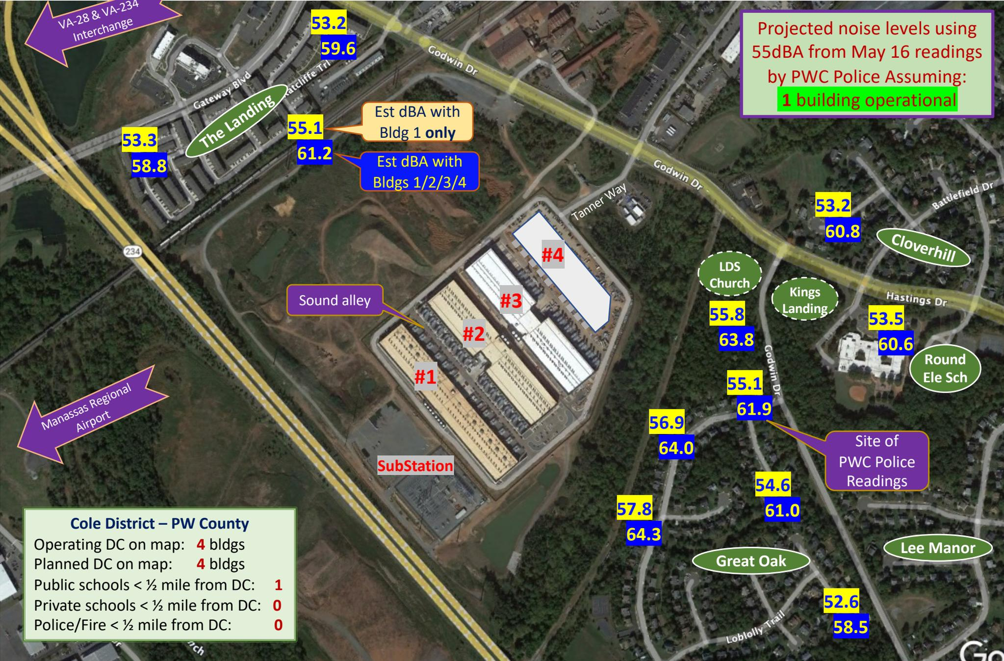
Projected noise levels using 55dBA from May 16 readings by PWC Police Assuming: **1 building operational**
