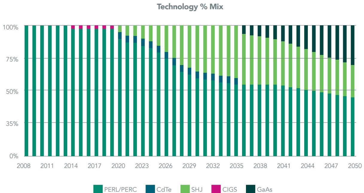
Crystalline silicon technology is poised to keep its dominant position till 2050, under the different hats of HJT & PERC and innovative new thin film technologies such as perovskite are expected to reach commercial
