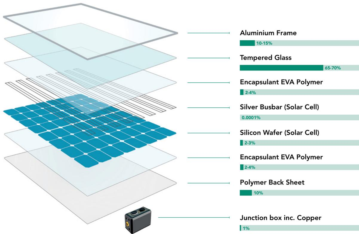
Each of the five energy technologies considered (PERC, SHJ, GaAs, CdTe and CIGS/CIS) were estimated to have constituent materials in varying proportions as shown in Figure 9 and this was used to model the material flows.
