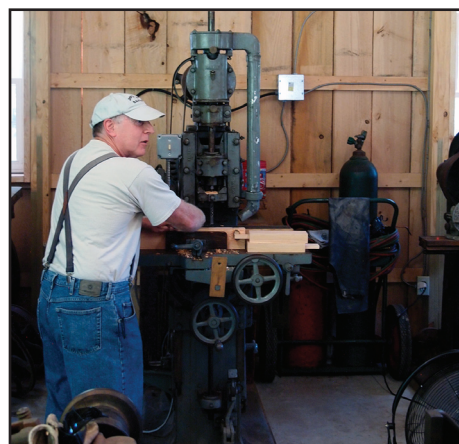
Blair Koberlein demonstrates the operation of an automatic mortise machine.
