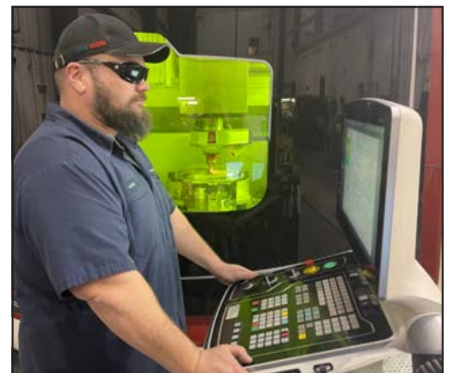
Machinist Supervisor Gene Steele operates the recently acquired 3D hybrid printing machine. With this initiative, ProEnergy is able to create critical parts for LM6000 gas turbines.
