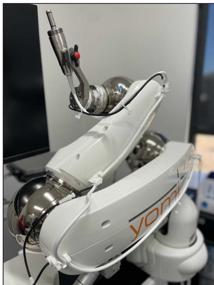
The YOMI robotic dental assistant uses 3D markers to precisely align Dr. Ehler's drill for perfect dental implant placement. PHOTO BY CHRIS HOWELL | DEMOCRAT
