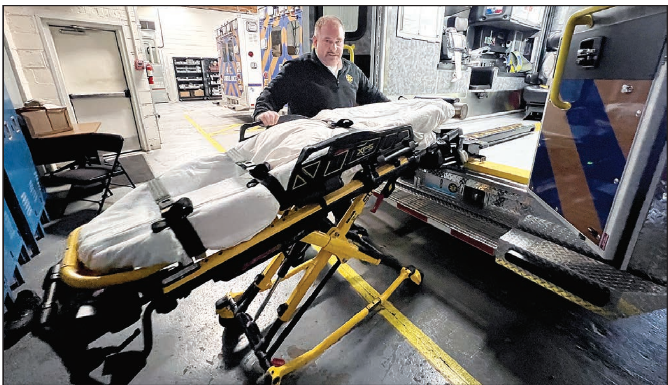
On Thursday, March 28, EMS Chief Roy Pennington shows how the bed in the new Pettis County Ambulance District Truck No. 8 is a power load bed, helping prevent back injuries for paramedics and EMTs. The new 2022 Ford E450 Super Duty was delivered to PCAD Headquarters on March 9.
