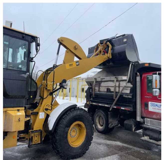
Kobe Slaughter loads salt into Chris Mittenberg's pilot truck Wednesday, Feb. 12. A brine liquid sprayed on the road salt makes it able to melt snow at lower temperatures.
